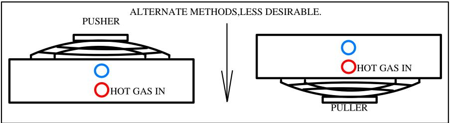
FOR MULTI-ROW COILS LIQUID LINE SHOULD ALWAYS RECEIVE AIR FIRST
